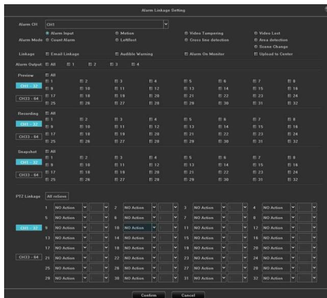
Figure10.19 Alarm Linkage
