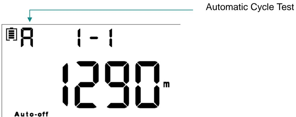
4. 2. 8 The unit starts to test 5s later. When the break is successfully repaired, a different value will be showed in the screen.
