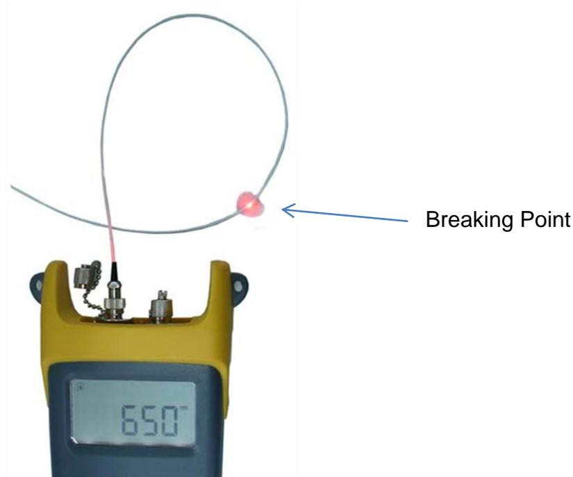
**Notice: Visible light source is harmful to the eyes. Do not look at the breaking point or end face of the tested fiber directly.**
