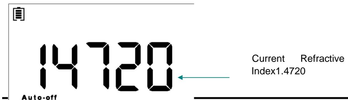
4. 2. 11 The refractive index ranges from 1.0000-2.0000. Press “▲/▼” keys to change the values and press “IOR” key to save and exit the changing mode.
