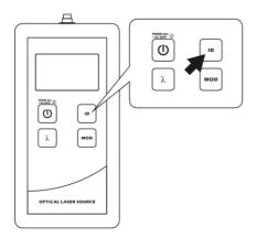
Press Button. the laser source will output with wavelength ID and LCD will display 'Id'. and if works with the paired power meter with WAVE ID function. the optical power meter will change to the same wavelength automatically.
