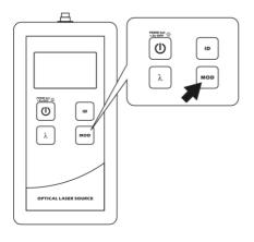
After pressing button, you can load a modulation current output laser.
