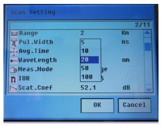
The "Setup of Pulse With" option has 11 predefined items in all, including 5ns, 10ns, 20ns, 50ns, 100ns, 200ns, 500ns, 1000ns, 5us, 10us and 20us. The setup is valid in the manual measurement mode only.
