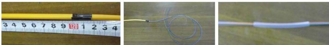
Pic 3:the length of stripped fiber cable    Pic4: fiber after stripping    Pic5: use EVA transparent tube to protect the stripped fiber
