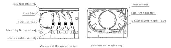
Pic1: The fiber route schematic diagram
