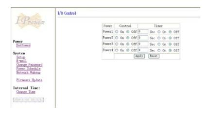
XL-IPM401 can control 4 outputs individually at the same time. User can choose power on or power off with an electrical outlet . User may fill in the corresponding columns with the delay time you wish in seconds, then choose the action after delay to be on or off.
