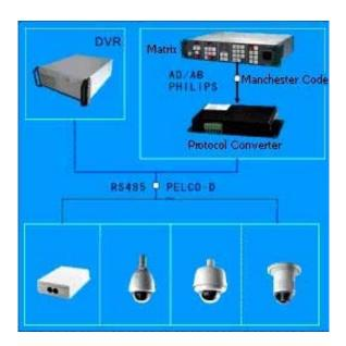
•The Matrix and DVR controls the terminal device.
