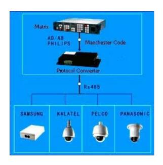
• The matrix controls the high speed dome and receiver with different protocol.
