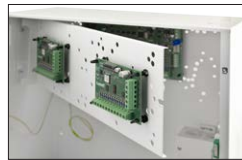
2 nd level - hinged mounting plate
