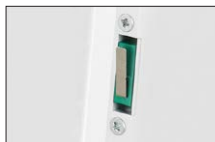
Tamper switch indicating enclosure opening - 1 piece
