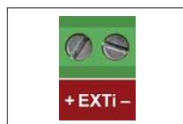
Input of external failure indication EXTi
