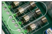
Fuse-protected outputs: glass fuse
