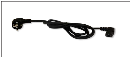
PSD13 Cable 230VAC 3x0.75mm 2 , 2m, CEE 7/7 (EF), IEC C13 angled plug
