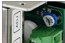
Potentiometer for output voltage adjustment
