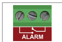
Relay type output of collective failure ALARM
