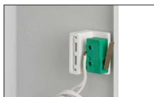
Tamper switch indicating enclosure opening
