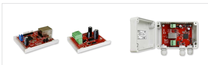
Interfaces (LAN, RS485) – only for EN54C...LCD series
