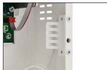
Tamper switch indicating enclosure opening - 1 piece
