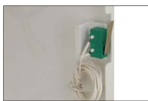
Tamper switch indicating enclosure opening - 1 piece
