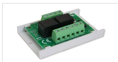
AWZ639 Technical outputs - relay (2x OC + 2x NO/NC/C)
