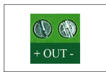
Power output terminals
