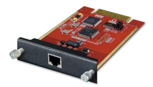
The E1/T1 module provided a RJ48 interface which could be configured to work in E1 (PRI-NET, PRI-CPE, R2, SS7 signaling) and T1 mode. You can install 2 E1/T1 modules on both IPX-2200 and IPX-2500. If it's going to be installed with other modules (IPX-21FO, IPX-21FS, IPX-21GS and IPX-21MA), it should be installed on Slot 2. And the E1/T1 module cannot be installed with BRI module like the IPX-2200 or IPX-2500.
