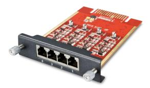
The IPX-21SL module provides 2 FXO and 2 FXS interfaces; it can be installed on both slots of the IPX-2100, IPX-2200 and IPX-2500. With the IPX-21SL module installed, it enables the IPPBX system with FXO to FXS lifeline feature. When there's power failure, you may still use the analog phone to make and receive phone calls.
