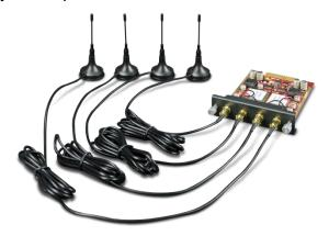
The IPX-21MA (WCDMA) module provides 4 GSM/3G voice channels; it can be installed on IPX-2100, IPX-2200 and IPX-2500 for making and receiving phone calls from the GSM/3G network. It is designed with SIM5320 series module for global market, the SIM5320 is a dual-band WCDMA and quad-band GSM engine that works on frequencies like UMTS 850MHz, UMTS 900MHz, UMTS 1900MHz, UMTS 2100MHz, GSM 850MHz, EGSM 900MHz, DCS 1800MHz and PCS 1900MHz.
