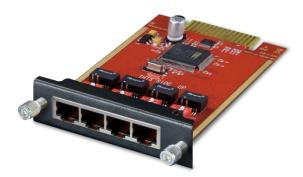
The IPX-21BR module provides 4 BRI interfaces which can be configured to work in NT or TE mode. It can be installed on IPX-2200 and IPX-2500 but not IPX-2100. Regarding the IPX-2200 and IPX-2500, only one 4BRI module can be installed. And if it's going to be installed with other modules (IPX-21FO, IPX-21FS, IPX-21GS, IPX-21MA modules), it should be installed in Slot 2. The IPX-21BR cannot be installed with E1 module like the IPX-2200 or IPX-2500.
