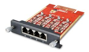
IPX-21FO module provides 4 FXO interfaces for connecting PSTN lines provided by the telecom. It can be installed on both slots of IPX-2100, IPX-2200 and IPX-2500 and provides maximal 8 FXO interfaces.
