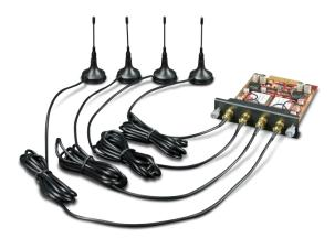
IPX-21GS module provides 4 GSM channels; it can be installed on IPX-2100, IPX-2200 and IPX-2500 for making and receiving phone calls from GSM network. It is designed with SIM900 for global market; SIM900 is a quad-band GSM engine that works on frequencies GSM 850MHz, EGSM 900MHz, DCS 1800MHz and PCS 1900MHz.
