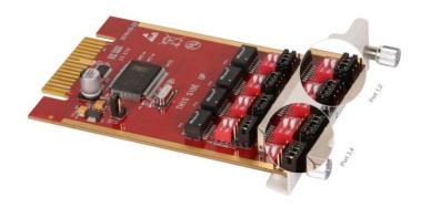
The jumpers for Port 1, 2 and Port 3, 4 are on different position. Attach the BRI lines to these ports and then configure BRI parameters.
