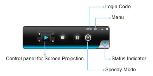
Figure 3-4 WPG Utility – Control Panel function Introduction
