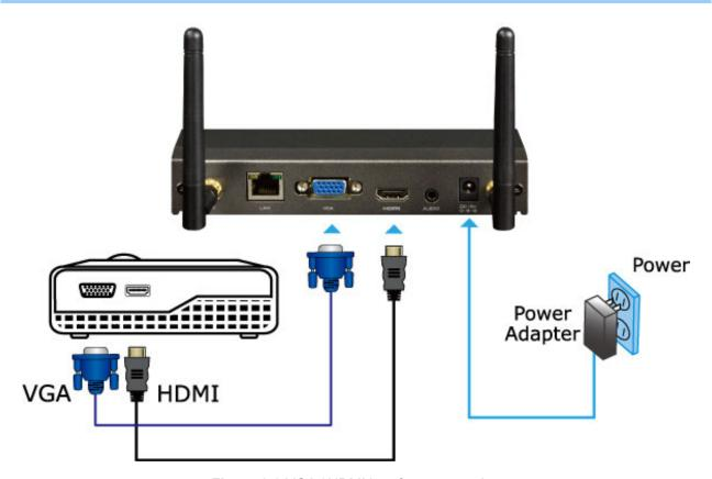
Figure 2-3 VGA / HDMI interface connection
