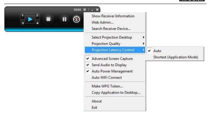
Figure 3-10 WPG Utility - Projection Latency Control
