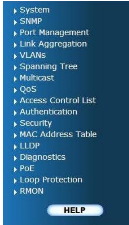
Figure 4-1-5: Managed Switch Main Functions Menu
