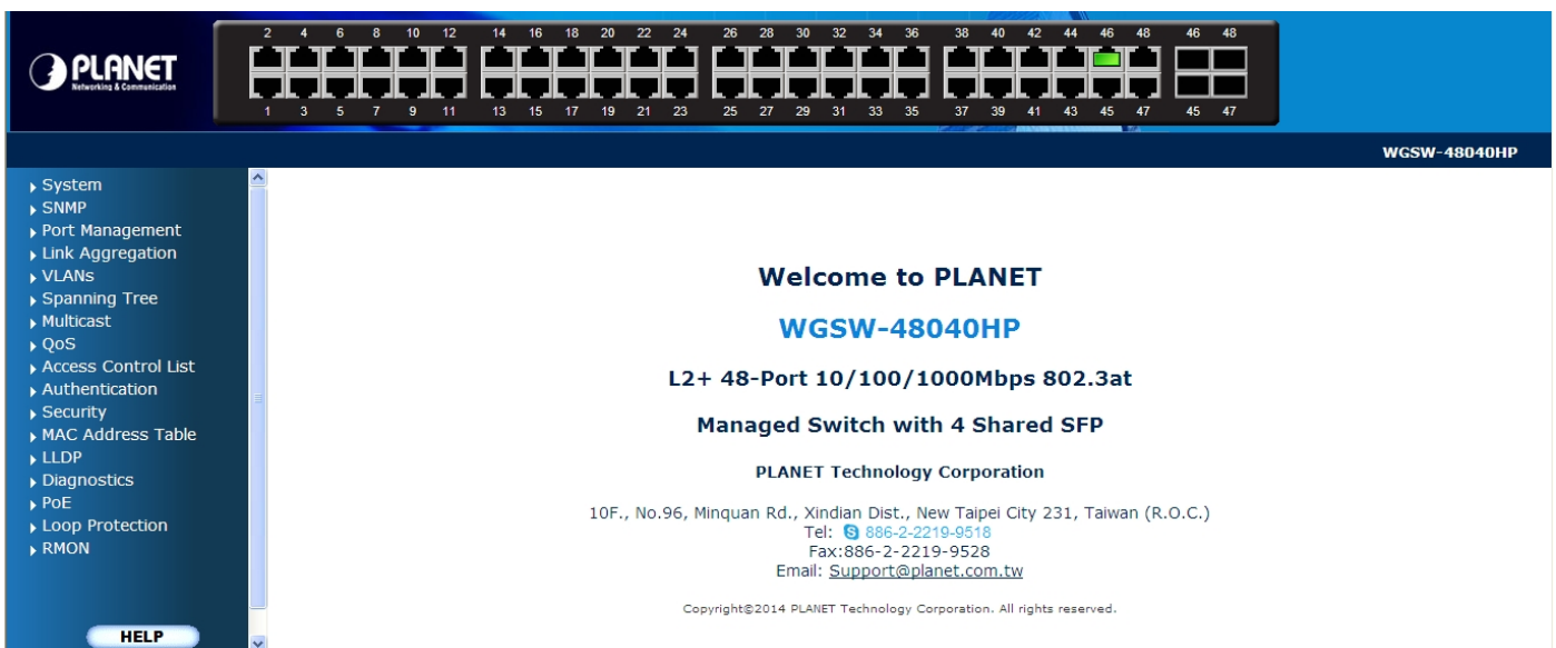
Figure 3-1-4: Web Main Screen of Managed Switch
