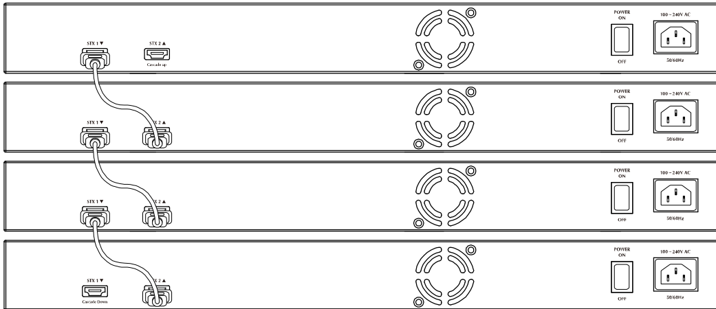
Figure 4-16-1 Chain Stack topology
