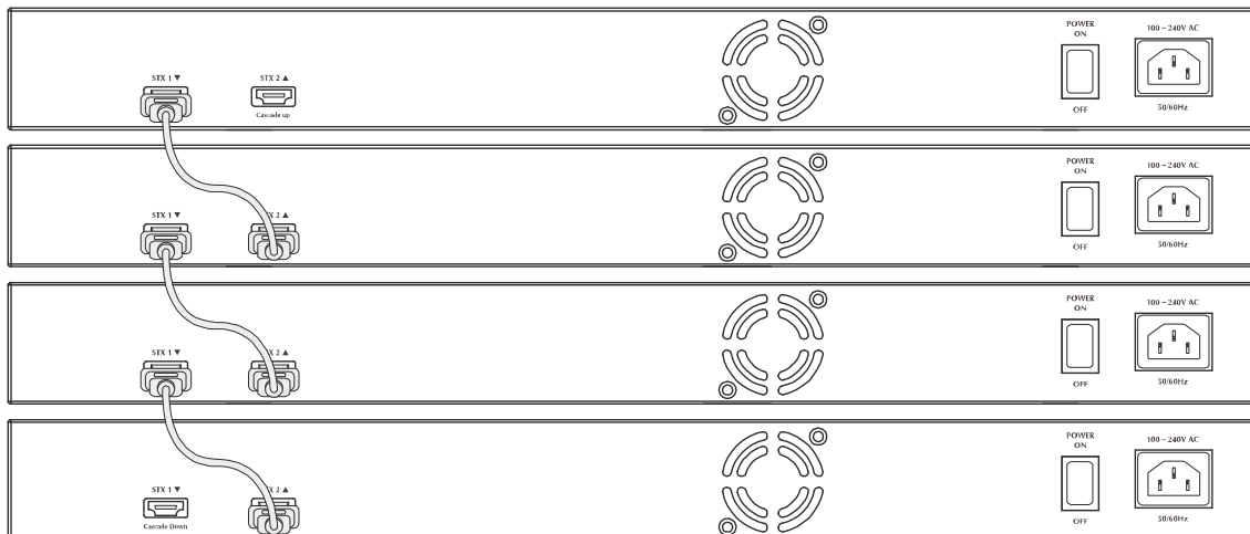
Figure 2-24 Chain Stack topology
