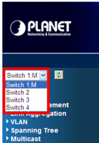
Figure 4-16-15 To manage the member switch
