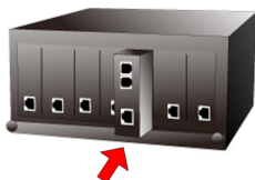
Figure 3-5: Insert a VDSL2 converter into an available slot
