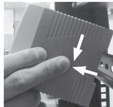
**Step 4:** Lightly press the button of DIN-Rail for remove it from the track.
