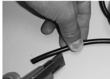
**Step 2:** Open the AC Power Cord Cable and there are 3 lines inside.
