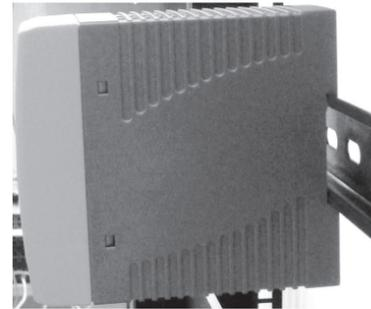
**Step 2:** Check the DIN-Rail is tightly on the track.
