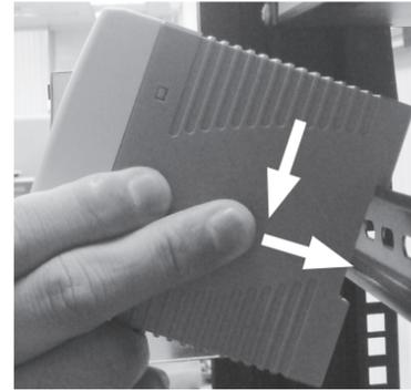
**Step 1:** Lightly press the button of DIN-Rail into the track.
