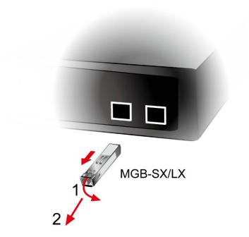
Figure 2-1-8 How to Pull Out the SFP Transceiver
