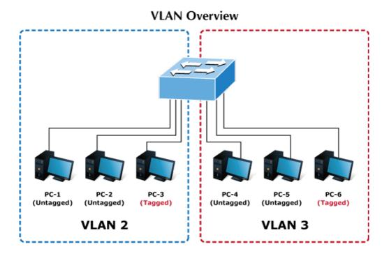
Figure 4-5-20 Two Separate VLAN Diagrams
