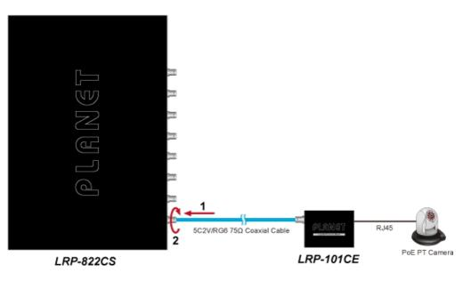
Figure 2-1-8 How to insert the coaxial cable from LRP Managed Switch
