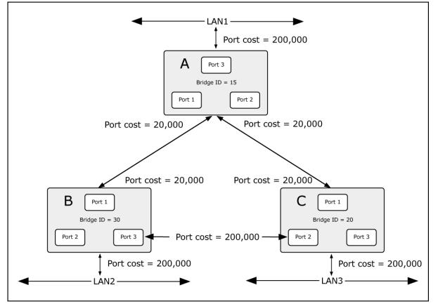
Figure 4-6-2 Before Applying the STA Rules
