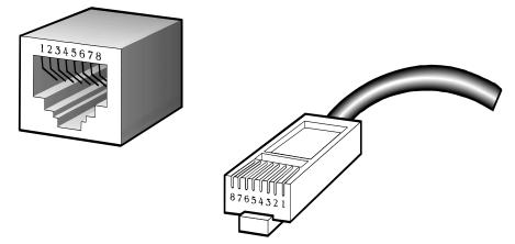
The standard RJ45 receptacle/connector
