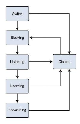
Figure 4-6-1 STP Port State Transitions
