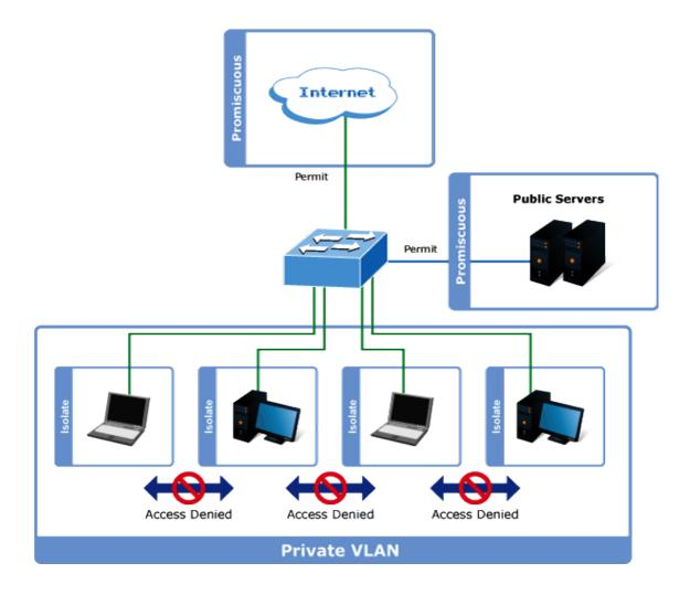
For protected port group to be applied, the LRP Managed Switch must first be configured for standard VLAN operation. Ports in a protected port group fall into one of these two groups:
