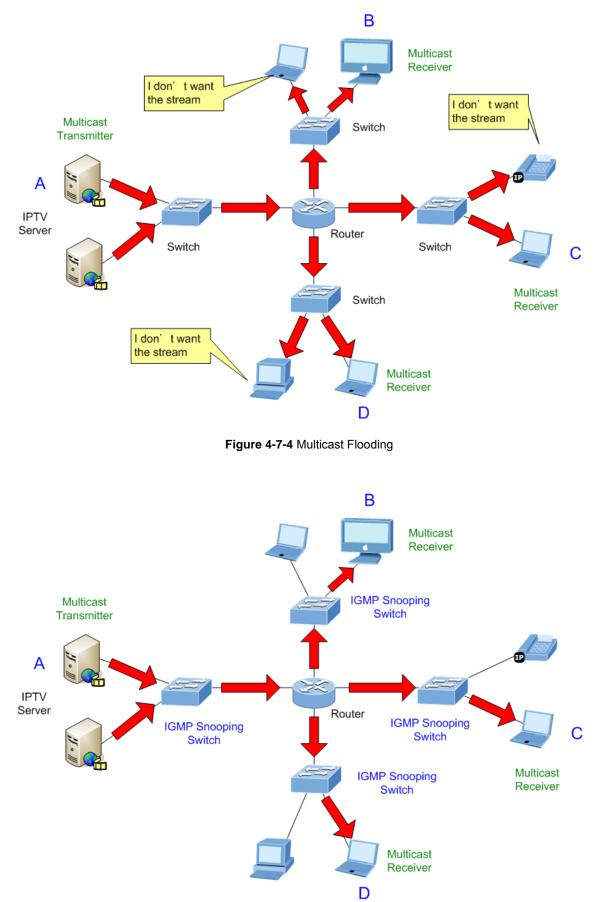
Figure 4-7-5 IGMP Snooping Multicast Stream Control
