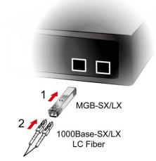
Figure 2-1-7 Plug in the SFP transceiver
