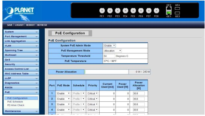
Figure 4-16-1: Power over Ethernet Status
