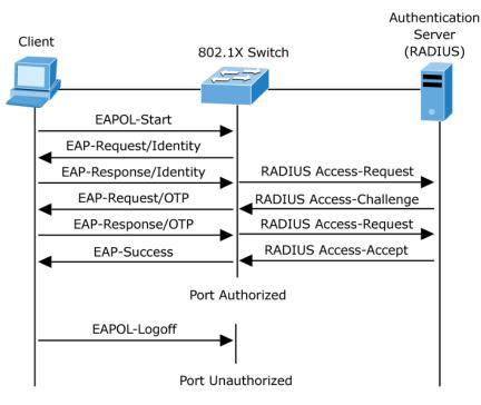
Figure 4-9-2 EAP Message Exchange
