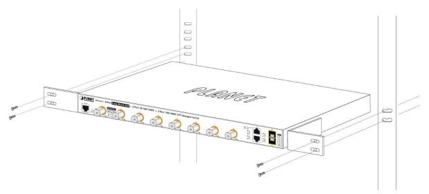
Figure 2-1-6 Mounting LRP Managed Switch in a Rack
