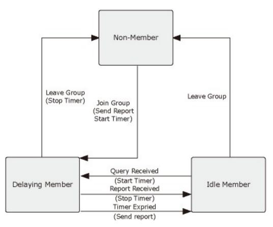
Figure 4-7-6 IGMP State Transitions
