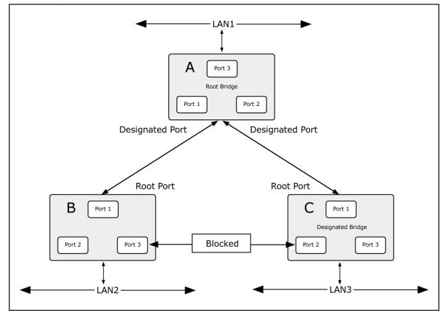
Figure 4-6-3 After Applying the STA Rules
