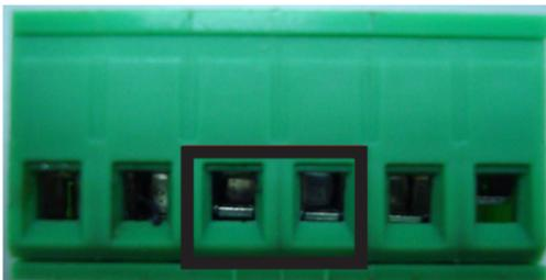
Insert the wires into the fault alarm contacts
