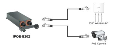
**Step 2:** The **"PoE-in-Use"** port is also the power injector which transmits DC voltage to the Cat5e/6 cable and transfer data and power simultaneously between the PSE and PD.
