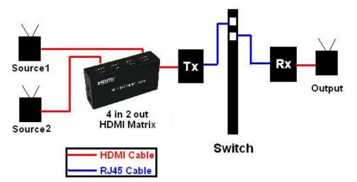
As you see, two sources connect to the input of HDMI matrix, and output to Tx, and then Tx and Rx all connect to the switch.
