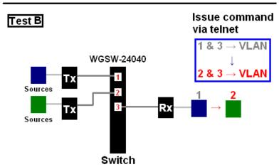
You can set up port-based VLAN for that Transmitter (IHD-200PT), and then for the receiver (IHD-200PR), You can just dynamically swap the receiver port to a different VLAN for video source change. You can swap VLAN via Web interface of the switch, say, WGSW-24040.
