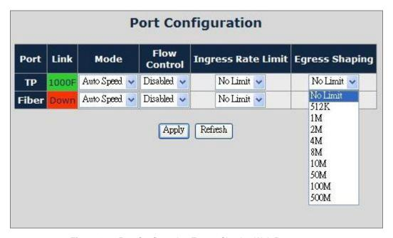
Figure 4-22 Port Configuration-Egress Shaping Web Page screen
