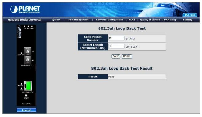
Figure 4-39 802.3ah Loop Back Test Web Page screen
