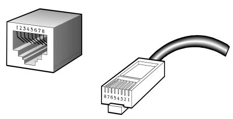
The standard RJ-45 receptacle/connector
