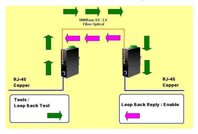
This function provides 802.3ah Loop Back Test of Industrial Managed Media Converter. Press the "Apply" button to run 802.3ah Loop Back Test and see the 802.3ah Loop Back Test Result of Industrial Managed Media Converter, also press the "Refresh" button to renew the Web screen. The screen in Figure 4-39 appears and Table 4-16 describes the 802.3ah Loop Back Test object of Industrial Managed Media Converter.
