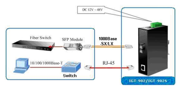
Figure 2-7 IGT- 902 / IGT-902T / IGT-902S / IGT-902TS stand-alone installation
