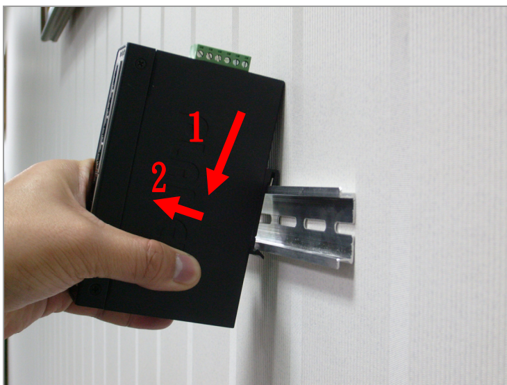
Figure 2-10 Remove Industrial Equipment in DIN-Rail mount.
