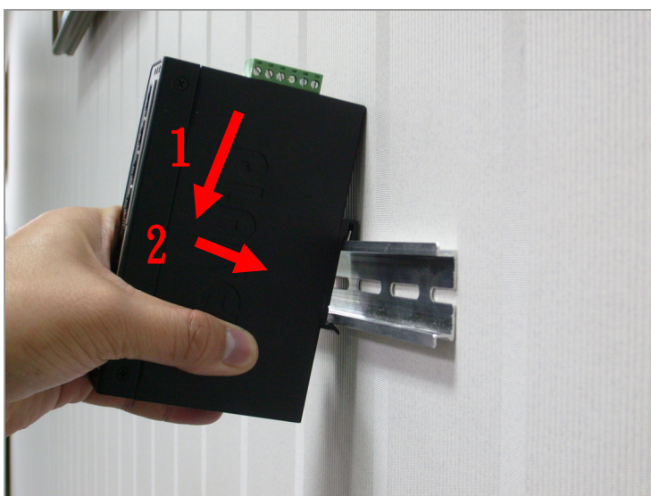
Figure 2-8 Install Industrial Equipment in DIN-Rail mount.
