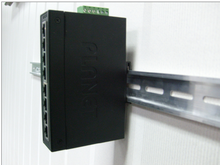
Figure 2-9 Industrial Equipment installed in DIN-Rail mount.
