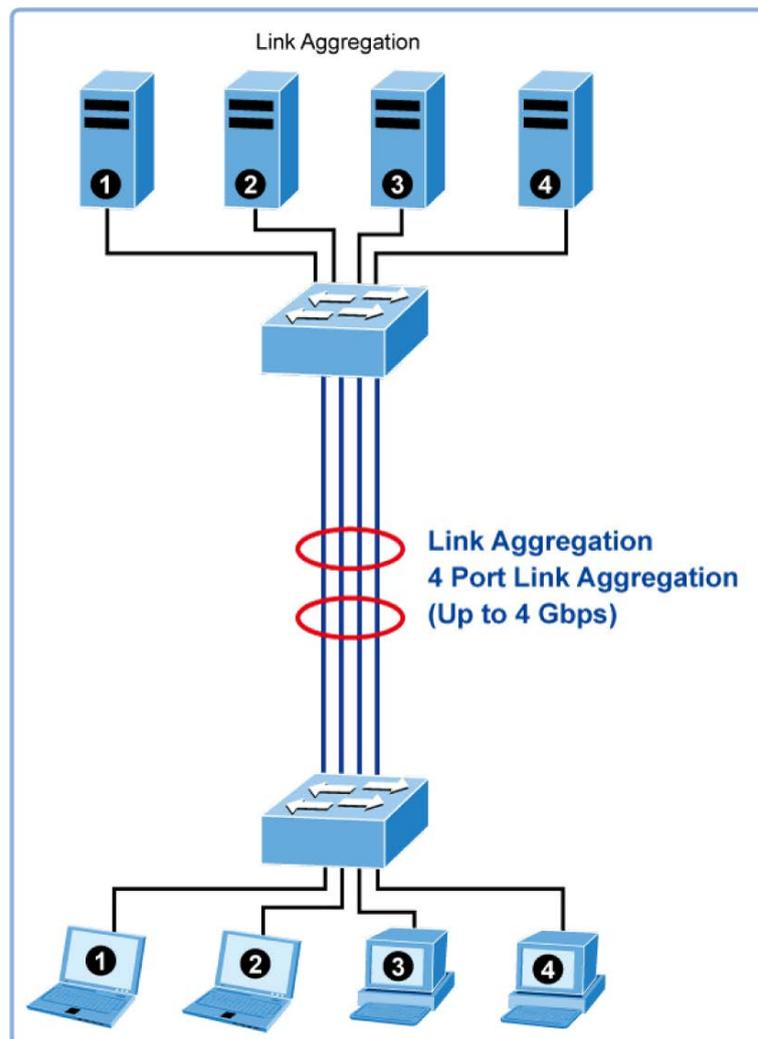
The **Link Aggregation Control Protocol (LACP)** provides a standardized means for exchanging information between Partner Systems that require high speed redundant links. Link aggregation lets you group up to eight consecutive ports into a single dedicated connection. This feature can expand bandwidth to a device on the network. LACP operation requires full-duplex mode, more detail information refer to the IEEE 802.3ad standard.
