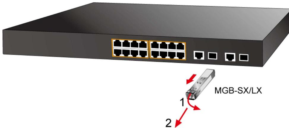
**Figure 2-8** How to Pull Out the SFP Transceiver
