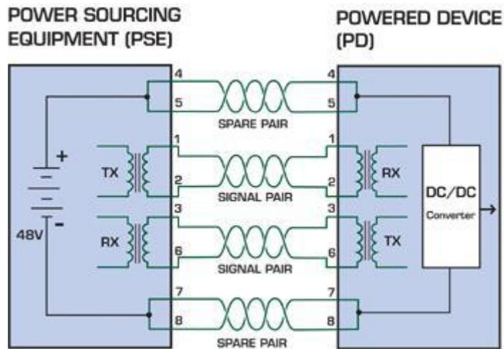
Figure 6-1: Power Supplied over the Spare Pins
