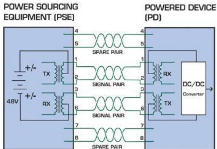
Figure 6-2: Power Supplied over the Data Pins
