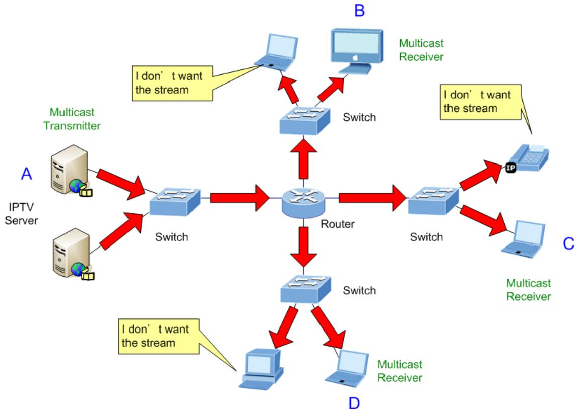
Figure 4-12-2 Multicast Flooding
