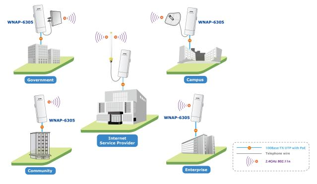
With built-in SMA-type Antenna connector and high output power with multiple adjust Tx controller, the WNAP-6305 provides higher coverage and longer distance wireless connection, and also allows CPE users to easily install and adjust the suitable value in appropriate locations. The WISP mode supported enables CPE users to connect to Internet via local WISP provider.
