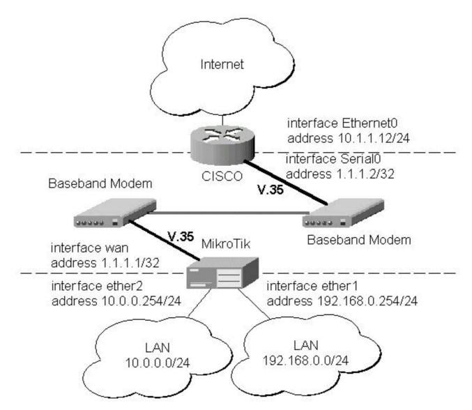
The driver for MOXA C101 card should be loaded and the interface should be enabled according to the instructions given above. The IP addresses assigned to the synchronous interface should be as follows:
