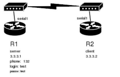
For a typical server setup we need to add one user to the R1 and configure the PPP server.
