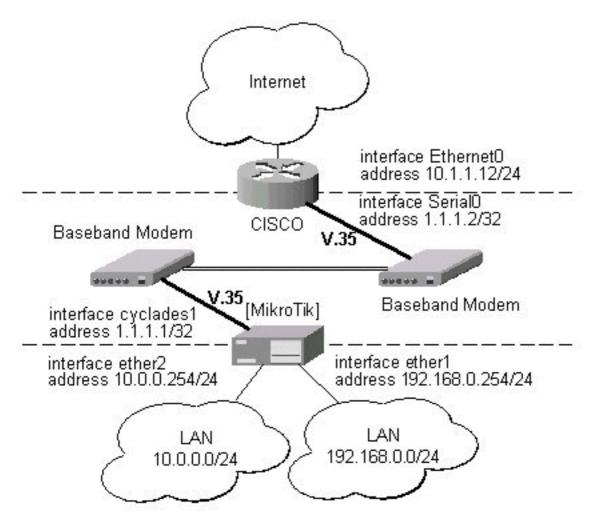
The driver for the Cyclades PC300/RSV Synchronous PCI Adapter should load automatically. The interface should be enabled according to the instructions given above. The **IP addresses** assigned to the cyclades interface should be as follows:
