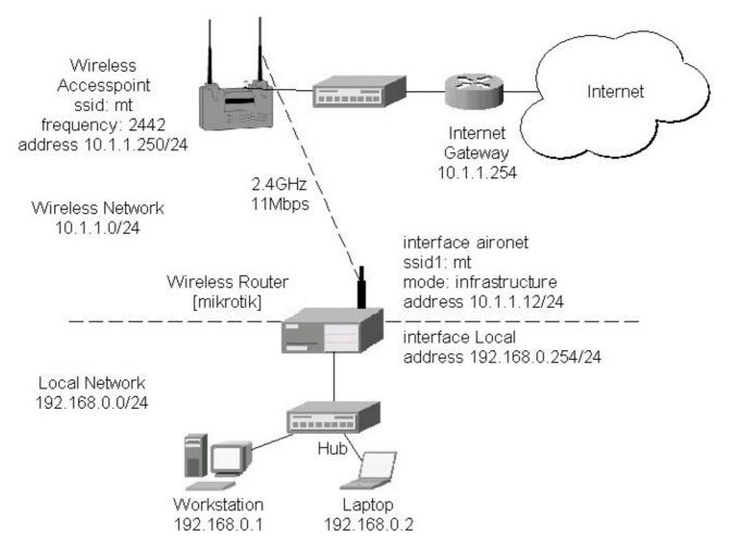
The access point is connected to the wired network's HUB and has IP address from the network 10.1.1.0/24.
