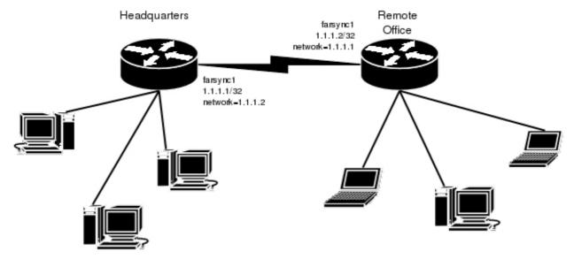
The default value of the property **clock-source** must be changed to **internal** for one of the cards. Both cards must have **media-type** property set to **X21**.
