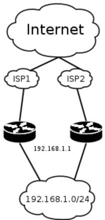
VRRP protocol may be used to make a redundant Internet connection with seamless fail-over. Let us assume that we have 192.168.1.0/24 network and we need to provide highly available Internet connection for it. This network should be NATted (to make fail-over with public IPs, use such dynamic routing protocols as BGP or OSPF together with VRRP). We have connections to two different Internet Service Providers (ISPs), and one of them is preferred (for example, it is cheaper or faster).
