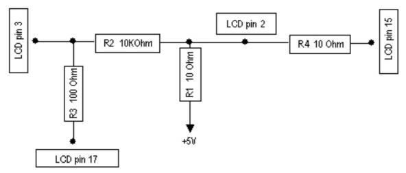
As there are only 16 pins for the PC1602 modules, you need not connect power to the 17th pin.
