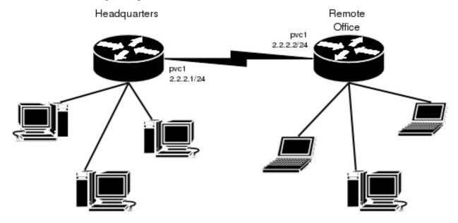
The default value of the property **clock-source** must be changed to **internal** for one of the cards. This card also requires the property **frame-relay-dce** set to **yes**. Both cards must have **media-type** property set to **X21** and the **line-protocol** set to **frame-relay**.
