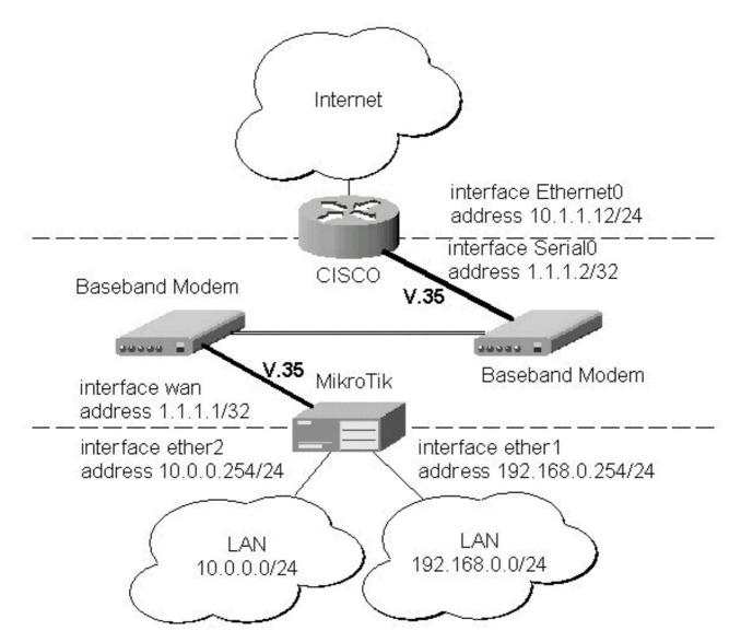
The driver for MOXA C502 card should be loaded and the interface should be enabled according to the instructions given above. The IP addresses assigned to the synchronous interface should be as follows:
