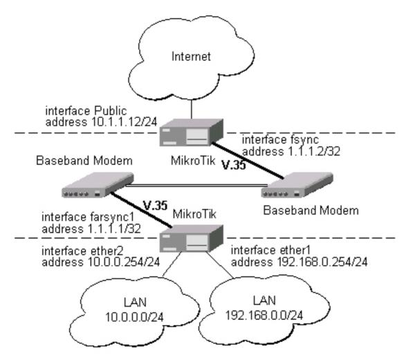
The interface should be enabled according to the instructions given above. The **IP addresses** assigned to the synchronous interface should be as follows:
