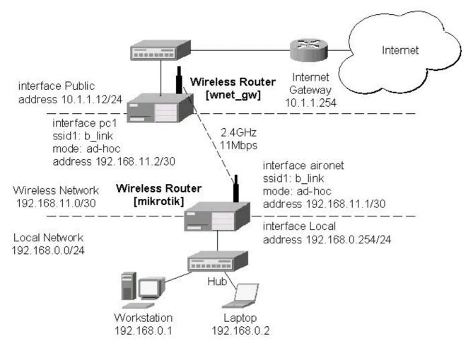
To establish a point-to-point link, the configuration of the wireless interface should be as follows:
