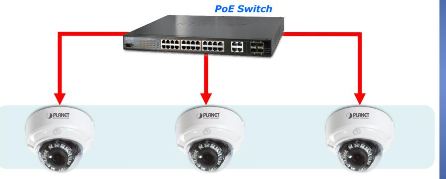
Compliant with IEEE 802.3af standard PoE interface. It can assist in locating cameras in places where there are no power outlets.
