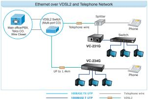
Refer to the following procedure to set up the VC-234G/VC-231G to IP DSI AM connection.
