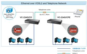
Refer to the following procedures to set up the VC-234G/VC-231G LAN to LAN connection.
