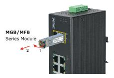
Figure 3-2: Pull Out from the Transceiver
